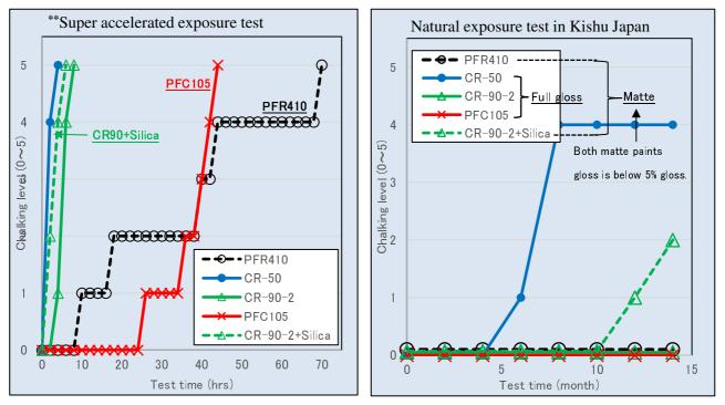
Chalking evaluation: No change = 0, 1, 2, 3, 4, 5 = Bad (JIS K5600-8-6) \*\*Super accelerated exposure test: Xenon arc + H2O2 spray
